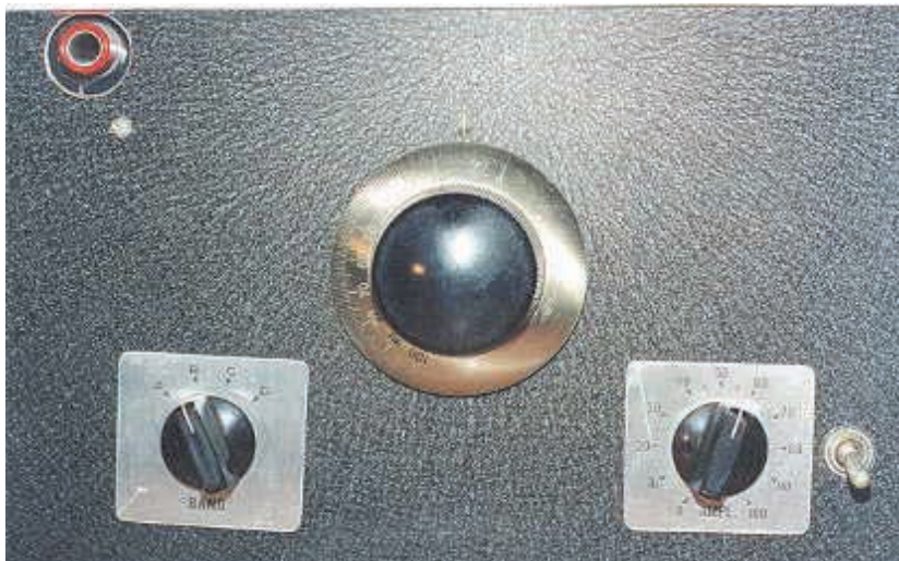
Front panel of the 1947 Rife Machine. The knob on the left changes the frequency band and the knob on the right changes the amplitude or power.
